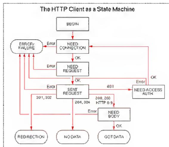
Figure 4: Http Client as a State Machine
